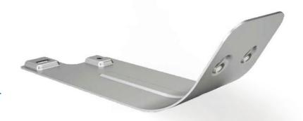
Riding on rough terrain? The brushed-aluminium sump guard is a must. It's designed to add a stylish layer of protection to the engine and lower frame rails.
