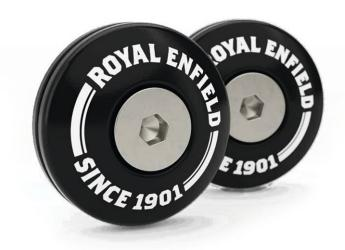
Subtly style your motorcycle with these handlebar finishers. They are machined from billet aluminium and anodized for a long life.
